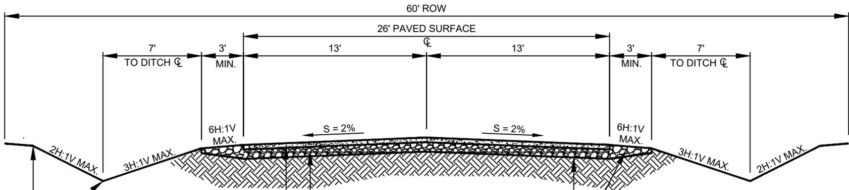
DITCH SHALL BE 1.5 FEET DEEP MIN. A DEPTH OF 5 FEET IS REQUIRED FOR CULVERT CROSSINGS. PLACE CHECK DAMS AT REGULAR INTERVALS FOR ROAD GRADES IN EXCESS OF 5%.
